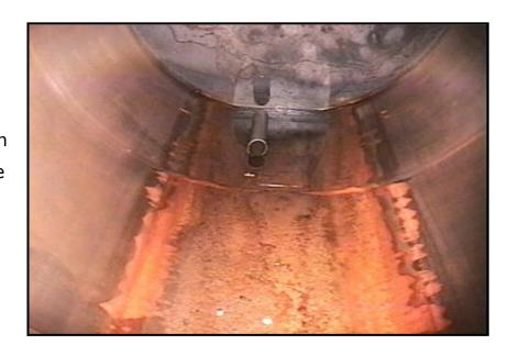
Tanknology's PetroScope system enables the thorough inspection of the interior of a UST, completely avoiding costly and dangerous excavation and manned tank entry.
