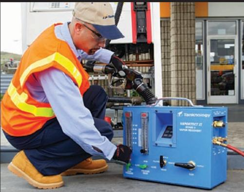
A Tanknology field technician performs a Stage II Vapor Recovery test on a fueling dispenser.
